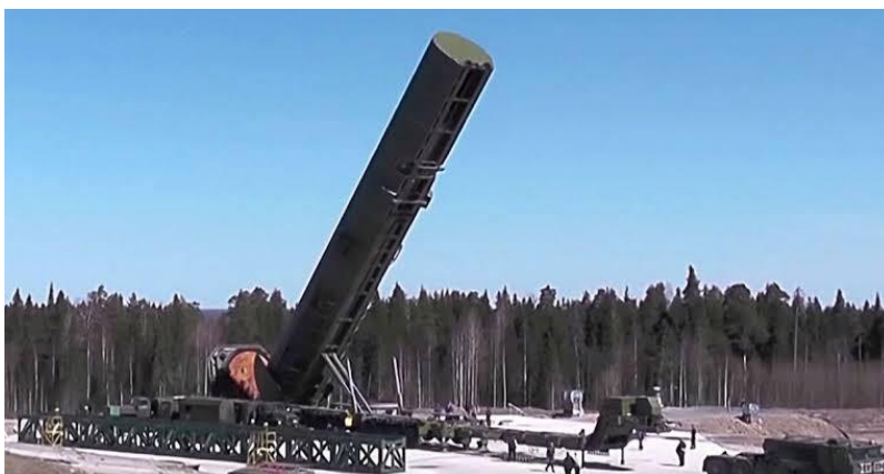
A Sarmat-associated transporter-erector raises a canister at a Russian test-and-deployment site. The Sarmat is emplaced in modified 15P718M silos and cold-launched by gas ejection before first-stage ignition.
