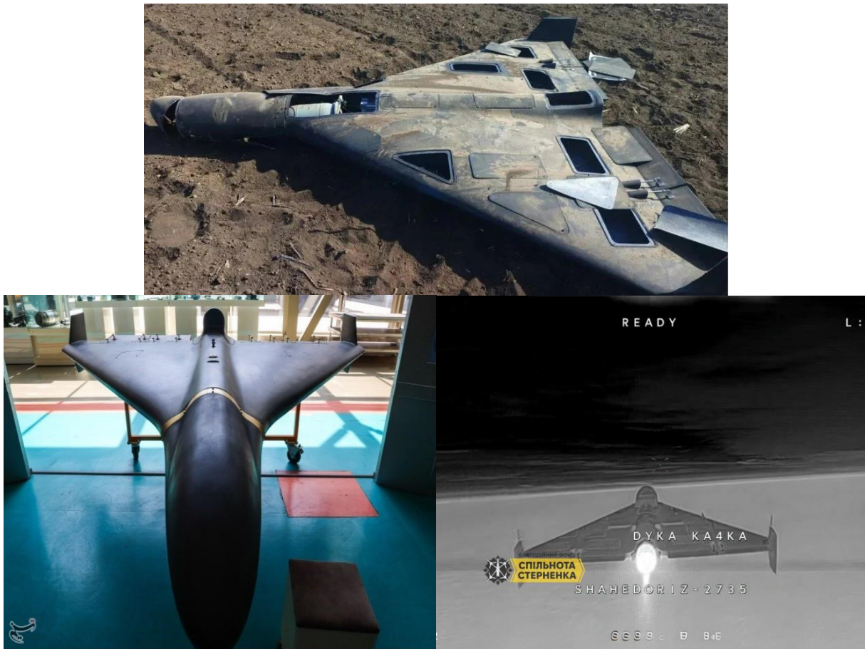
Figure 1. Recovered wreckage of a Russian Geran-2 (Iranian Shahed-136) loitering munition downed over Ukraine, showing the composite delta-wing airframe and rear pusher-propeller mount. (Open-source imagery.), Russian Geran-3, and captured image of an aerial Geran-4.
