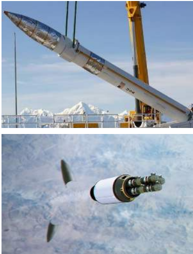
Top: GBI being lowered into its silo Bottom: MOKV Concept Art
