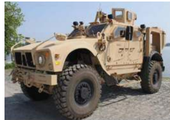
M-ATV with Underbody Improvement Kit (UIK)
