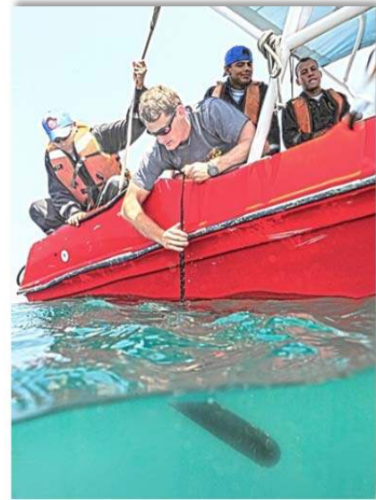
A U.S. Navy Diver lowers a side-scan sonar with the help of Colombian divers during Navy Dive-Southern Partnership Station 2012, off the coast of Colombia. (U.S. Navy photo by Petty Officer 2nd Class Kathleen A. Gorby)
